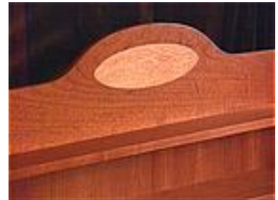
The maple inlay was added using a hand-held router and specialized router-inlay kit.
